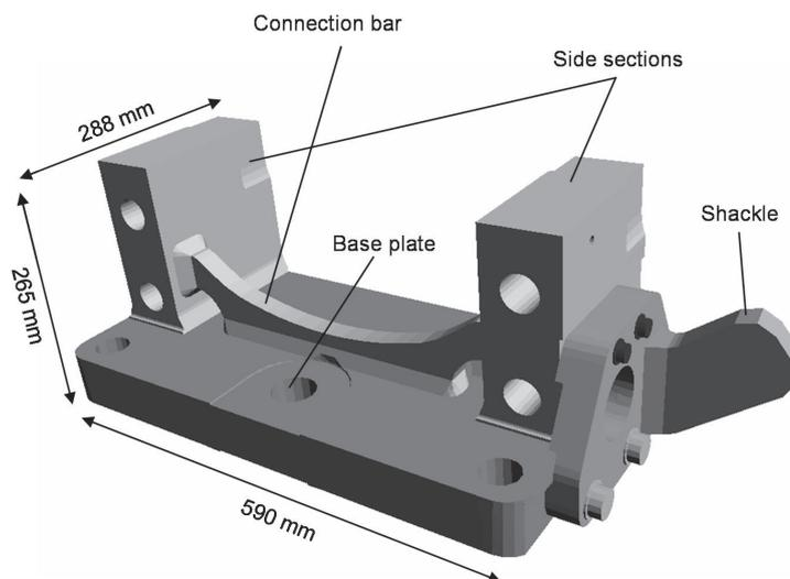
Fig. 2. Engine cradle (machined) with base plate, side sections left/right, each with two through-holes as well as welded brace and right shackle which is screwed on
