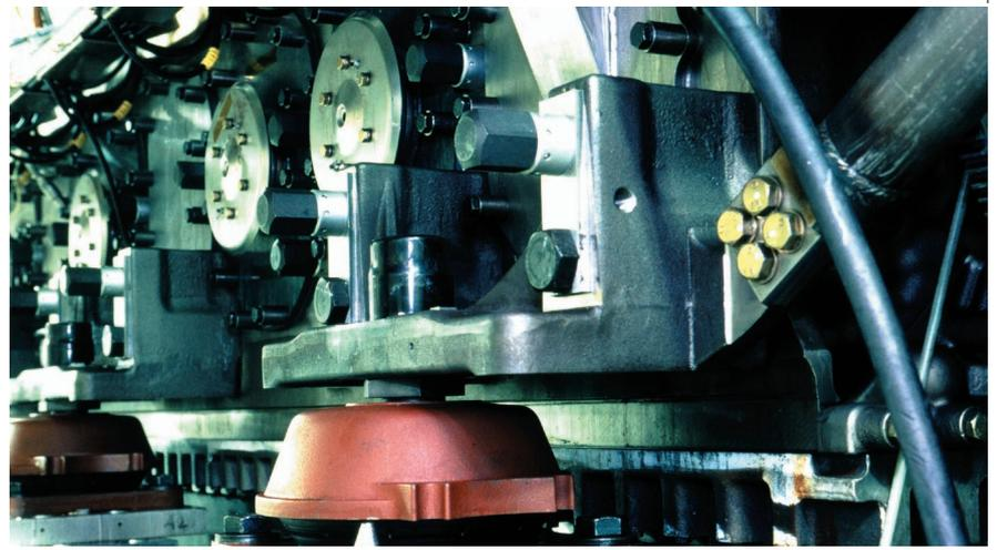
Engine cradle for the high performance Diesel motor made from ADI (model MTU Friedrichshafen Ltd, series BR.8000)
