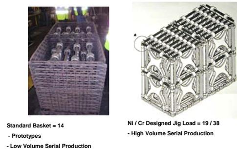
**Figure 8: Furnace loading jigs**
