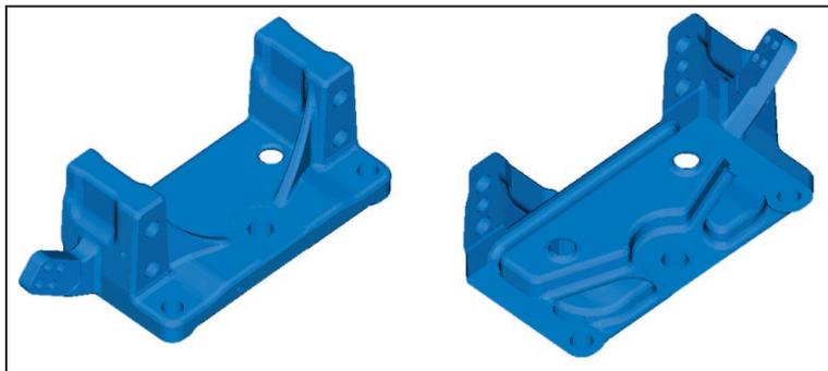
Fig. 4. Single component motor cradle cast using ADI with left founded shackle; (left) view from above with webs between the side sections and the bearing connection. The side sections have pockets on both sides; (right) view from below with wall thickness reduced base plate and ridge structure for rigidity
