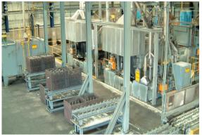
Fig. la. Purpose built furnaces for production of ADI and CADI. This facility at ADI Treatments Ltd operates the largest furnace of its kind in commercial use, accommodating parts up to 18m diameter
