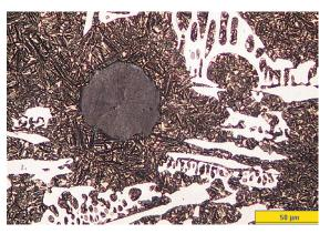
Fig. 3. A typical CADI microstructure showing carbide and spheroidal graphite, dispersed in an ausferrite matrix and austempered at 370°C
