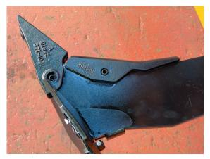
Fig. 4. Ground engaging components on the SIMBA Solo subsoiler. The CADI shin part bearing the company logo is appositely positioned behind the white iron tip. Courtesy SIMBA International, www.simba.co.uk
