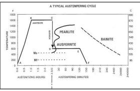
Fig. 2. A schematic representation of the CADI heat treatment cycle
