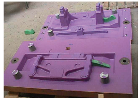
Fig. 7. Moulding plates for the broad engine cradle made from ADI with interchangeable shackle (right or left)
