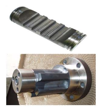
Figure 12: Mini Excavator rack and pinion
